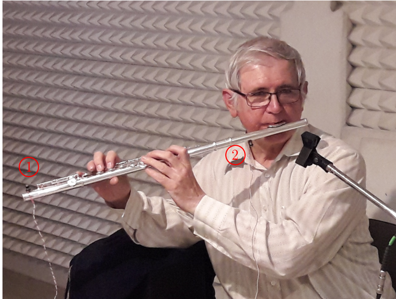
Figure 2: Positions of the accelerometers on the flute
