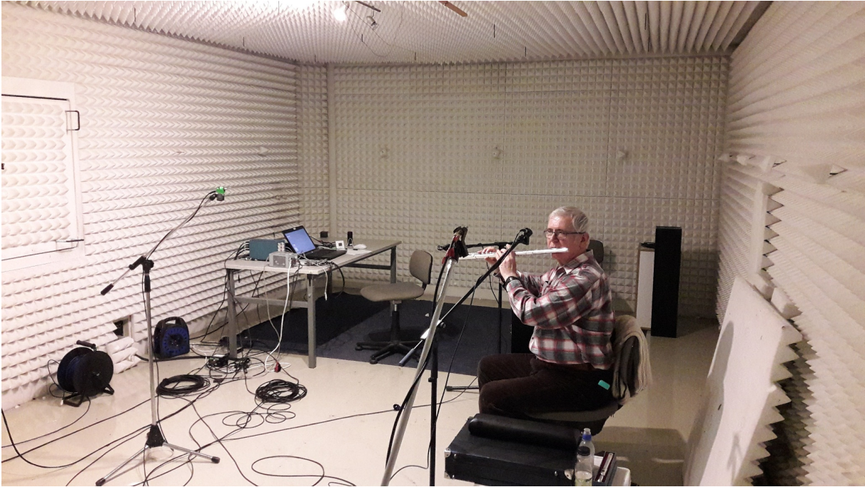
Figure 1: Measurement arrangement in the semi-anechoic chamber
